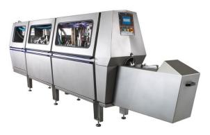
VISIOMASTER - yet another option, which by its purpose inspects the processed fish, and automatically determines whether it is accepted for further processing or needs to be checked manually.
